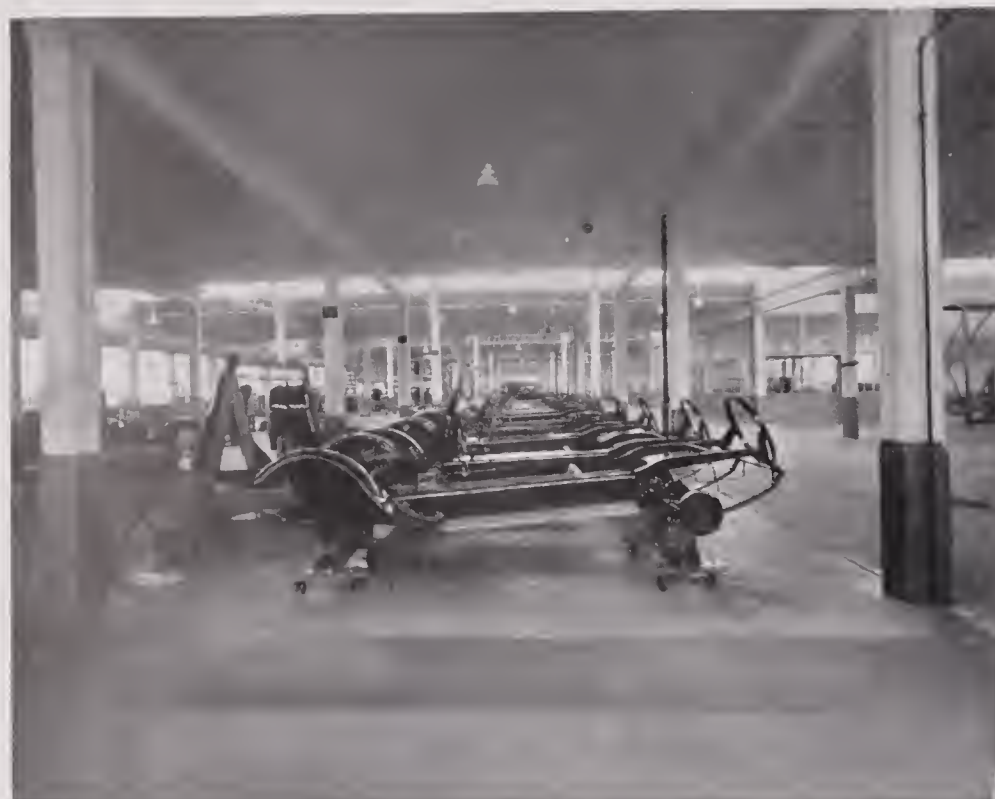
MODEL 250'S IN EARLY STAGE OF ASSEMBLY
